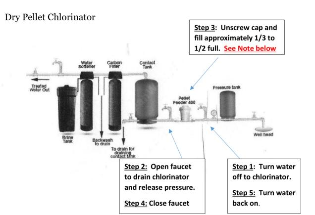
**Note:** After filling the chlorinator with pellets, please check to be sure the threads on the cap are free from powder residue before screwing the cap back on.
